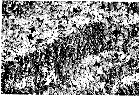
Fig. 5. Polarized light micrograph showing prior \beta grain size limiting extent of surface slip. Electropolished short transverse tensile test piece cut from the 2\frac{1}{2} in thick forged and annealed Ti-6Al-4V bar. Stress axis shown by arrow. X330
