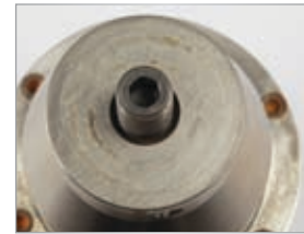
Fretting corrosion on horn/ booster interface
