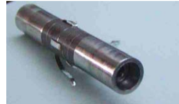
40 kHz test transducer with Stainless steel end masses
