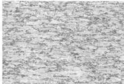
Alpha Case in Ti 6Al-4V
