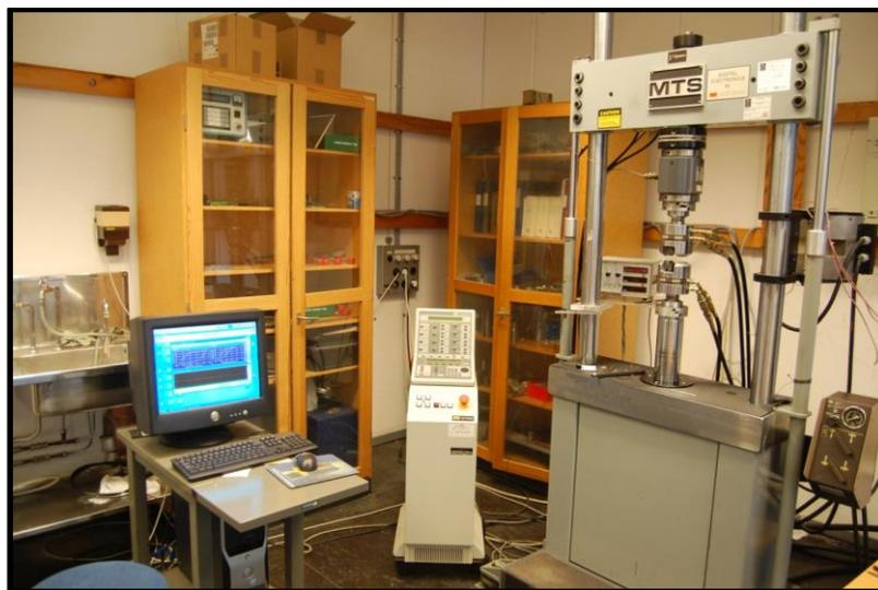
**Figure 3.8** MTS Ramen machine used for tensile testing and fatigue testing.
