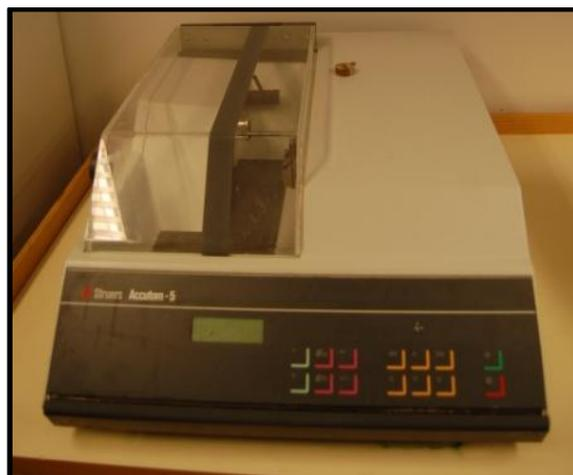
**Figure 3.4** Struers Accutom-5 machine used for cutting.
