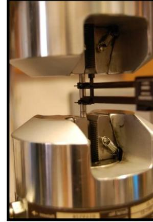
**Figure 3.11** Extensometer used to measure the deformation in the tensile test.
