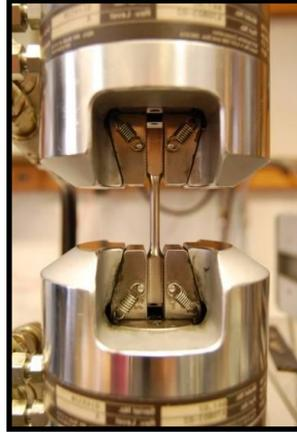
**Figure 3.10** Sample ready for the test.
