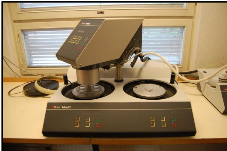
**Figure 3.6** Struers Rotopol-2 used for grinding and polishing.
