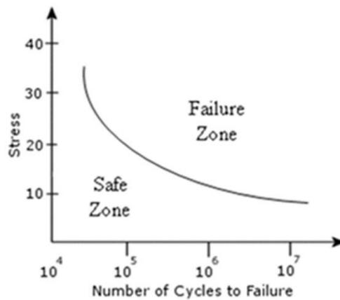
**Figure 2.2** Typical  $S$ - $N$  curve of a material.
