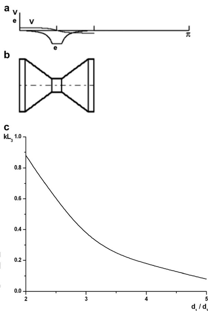
Fig. 6. Symmetrical spool-shaped horn is shown with  $d_1 = d_5$ ;  $kL_1 = kL_5 = 0.1$ ;  $kL_3 = kL_4 = 0.5$ , along with (a) the distribution of the oscillatory velocity,  $V$ , and strain,  $e$ , along the horn; (b) drawing of the horn; (c) plot of the distribution of the horn's parameters.
