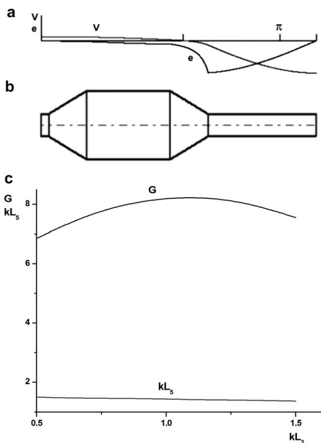
Fig. 5. Barrel horn is shown with  $d_1 = d_5$ ;  $d_3/d_1 = 3.0$ ;  $kL_1 = 0.1$ ;  $kL_2 = kL_4 = 0.5$ , along with (a) the distribution of the oscillatory velocity,  $V$ , and strain,  $e$ , along the horn; (b) drawing of the horn; (c) plot of the distribution of the horn's parameters.
