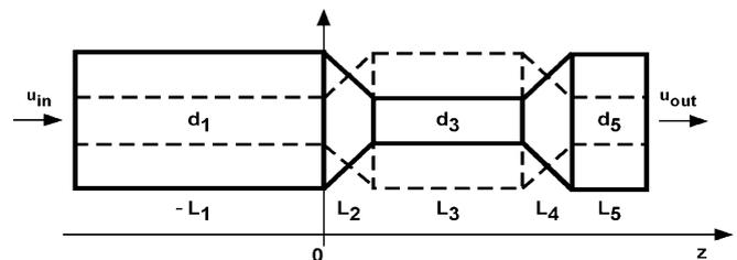
Fig. 2. Schematic defining the parameters of a five-element matching horn is shown. The horn having  $d_1/d_3 > 1$  is shown by a solid line, and the horn with  $d_1/d_3 < 1$  is shown by a dotted line. Parameters  $L_1$ – $L_5$  correspond to the lengths of each element.
