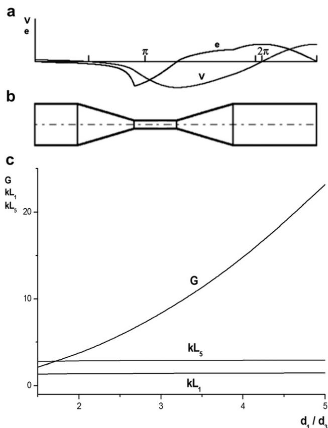
Fig. 7. Barbell-shaped horn is shown with  $d_1 = d_5$ ;  $kL_1 = kL_3$ ;  $kL_2 = kL_4 = 0.5$ , along with (a) the distribution of the oscillatory velocity,  $V$ , and strain,  $e$ , along the horn; (b) drawing of the horn; (c) plot of the distribution of the horn's parameters.
