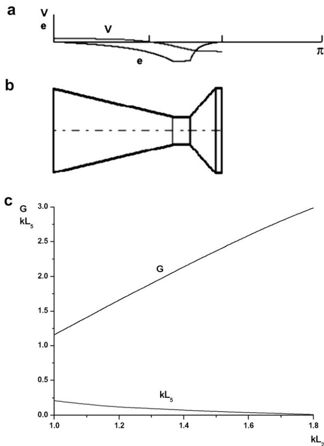
Fig. 3. Conical-cylindrical horn is shown with  $d_1 = d_5$ ;  $d_1/d_3 = 3.0$ ;  $kL_1 = 0$ ;  $kL_3 = 0.2$ ;  $kL_4 = 0.3$ , along with (a) the distribution of the oscillatory velocity,  $V$ , and strain,  $e$ , along the horn; (b) drawing of the horn; (c) plot of the distribution of the horn's parameters.
