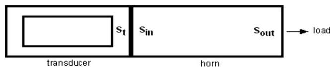
Fig. 1. General schematic is shown, describing matching between an electromechanical transducer and a load achieved by using an acoustic rod horn of an arbitrary shape.  $S_{in}$  and  $S_{out}$  are, respectively, the input and the output cross-sections of the acoustic horn;  $S_t$  is the output cross-section of the electromechanical transducer.
