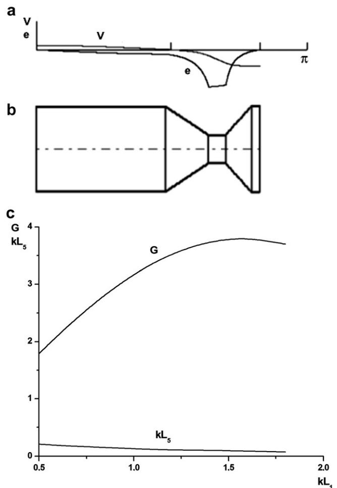
Fig. 4. Stepped horn is shown with  $d_1 = d_5$ ;  $d_1/d_3 = 3.0$ ;  $kL_1 = 0.5$ ;  $kL_3 = 0.2$ ;  $kL_4 = 0.3$ , along with (a) the distribution of the oscillatory velocity,  $V$ , and strain,  $e$ , along the horn; (b) drawing of the horn; (c) plot of the distribution of the horn's parameters.
