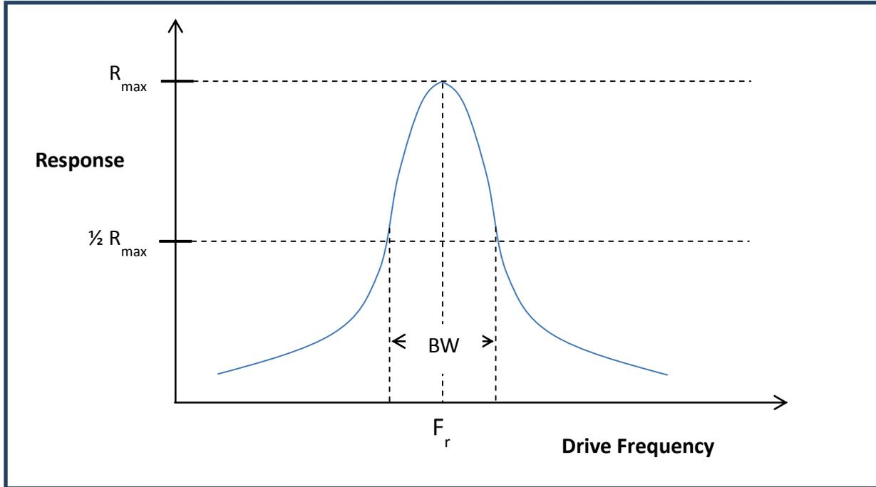
**Figure 8: Response Curve for a Damped and Driven System.** The response rises to a maximum at the resonant frequency  $F$ . The difference in frequency between the maximum and the point where the response drops to one half of the maximum response defines the bandwidth,  $BW$ . The system's quality factor  $Q = F_r/BW$ .
