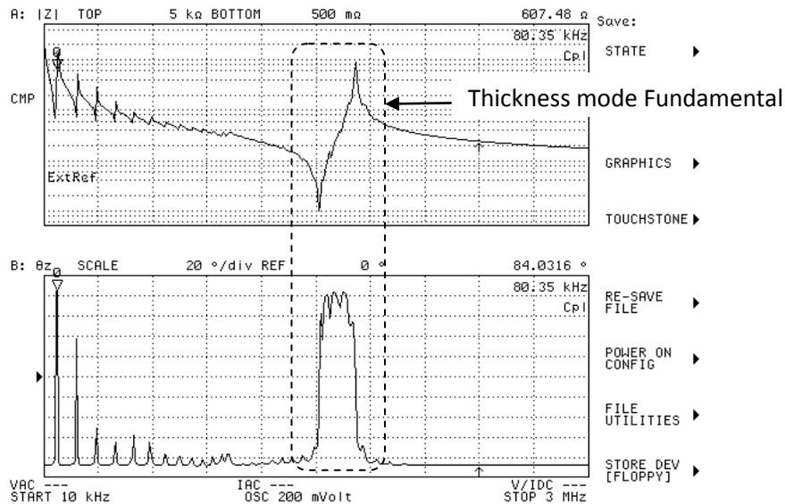
**Figure 5: Fundamental Thickness Mode Resonance.** The thickness mode resonance is much wider and stronger than the radial mode harmonics.
