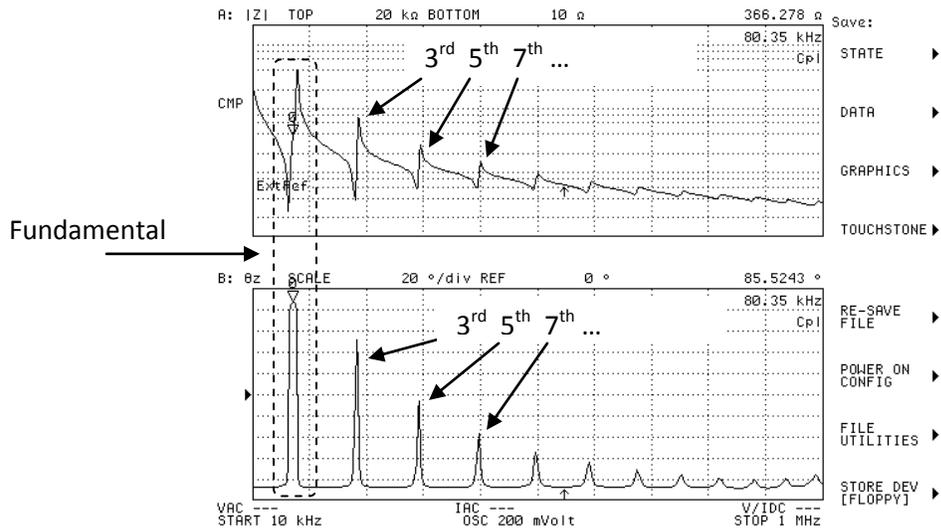
**Figure 4: Radial Frequency Harmonics.** The fundamental resonance is followed by a series of odd harmonics at progressively higher frequencies. The strength of the harmonic and the spacing between the resonances decreases as the order increases.
