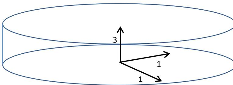
**Figure 2: Axes in a piezoceramic disk.** For piezoceramic disks as shown in Figure 1, the two axes 1, which are in the plane of the disk, are equivalent. The axis 3 is perpendicular to the plane of the disk.
