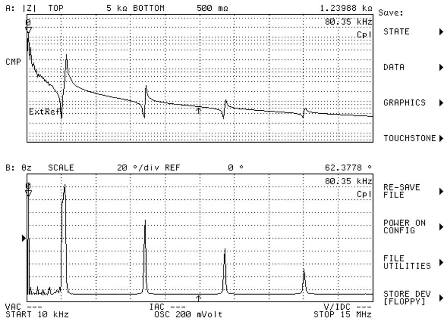
**Figure 7: Thickness Mode Harmonics.** The 3<sup>rd</sup>, 5<sup>th</sup>, and 7<sup>th</sup> harmonics are progressively weaker than the fundamental thickness mode.
