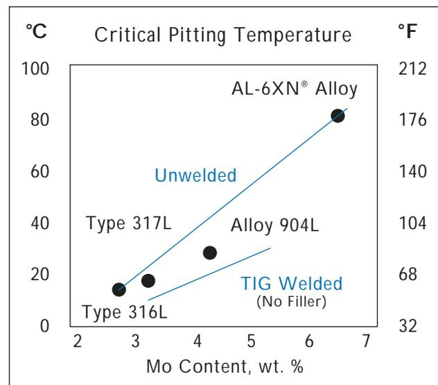
**FIGURE 4: Critical pitting temperatures in ferric chloride solutions.<sup>10</sup>**
