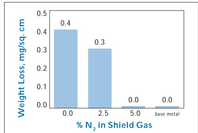
**FIGURE 28:** Effect of GTA weld shielding gas composition on the crevice corrosion resistance of autogenous welds in AL-6XN<sup>®</sup> alloy tested per ASTM G-48B at 35°F.
