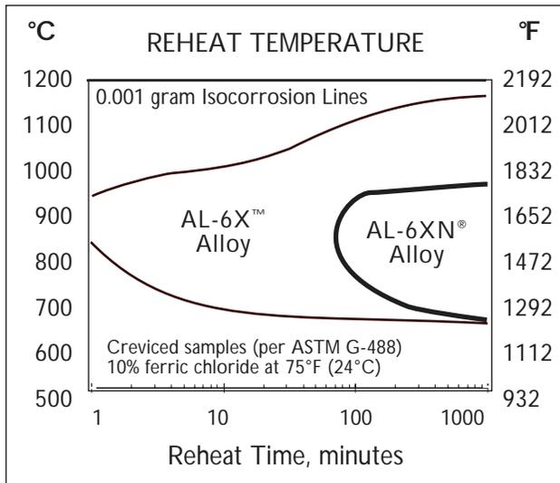
**FIGURE 1:** Time-temperature-corrosion curves for heat-treated samples (0.001 gram weight).
