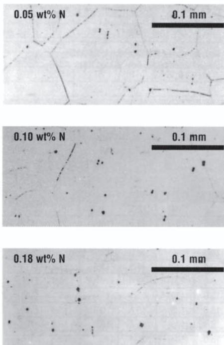
**FIGURE 2:** Effect of nitrogen on sigma phase precipitation.
