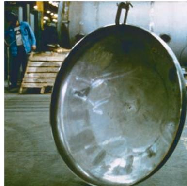
**FIGURE 26:** A warm formed vessel head of AL-6XN® plate.
