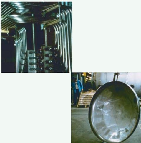
resistant than Type 316 and somewhat better than Alloy 904L. The performance of AL-6XN alloy is similar to that of the more costly materials that are often used in sulfuric acid, such as Alloy 20 and Alloy 825. AL-6XN alloy also has excellent resistance in sulfuric acid contaminated by chlorides (Figure 12).
