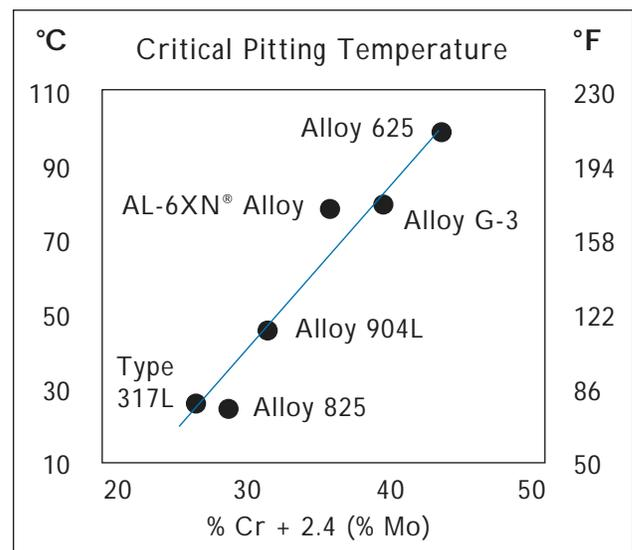
**FIGURE 5: Critical pitting temperatures in an acidic mixture of chlorides and sulfates.<sup>14</sup>**
