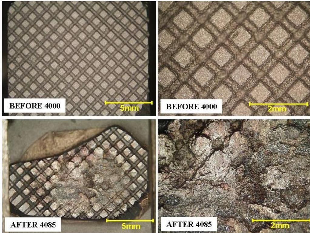
**Figure 31: W-25Re anvil wear during weld trials 4000-4085, anvil surface fractured and re-brazed during trials**
