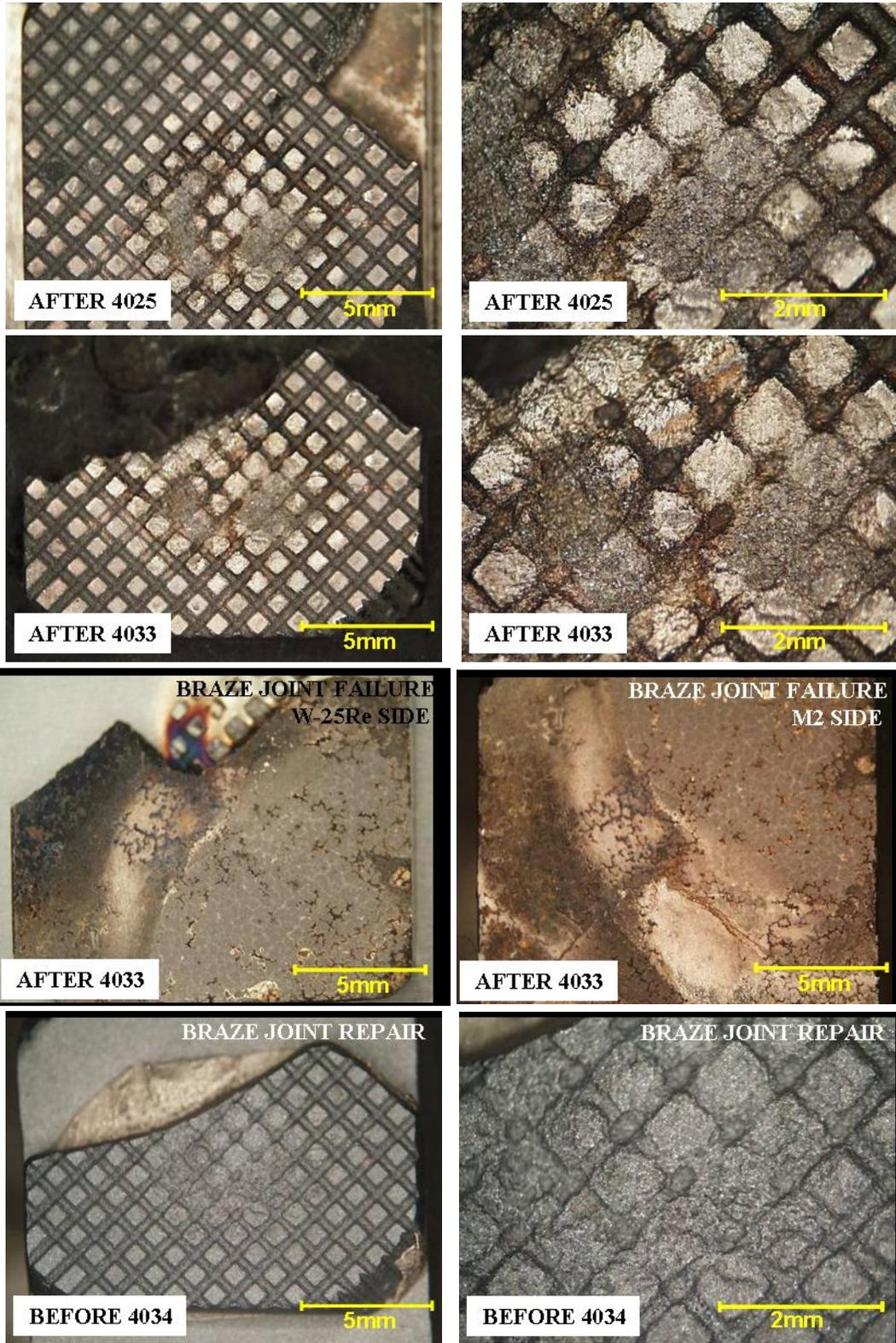
Figure 125: W-25Re anvil during SS 304 weld trials 4025-4034
