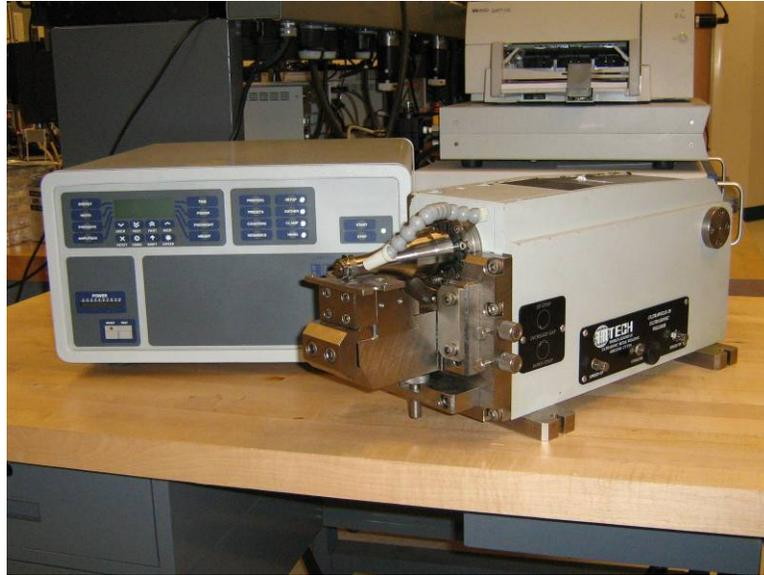
**Figure 6: AmTech Ultraweld 20 Lateral-drive Ultrasonic Spot Welder**
