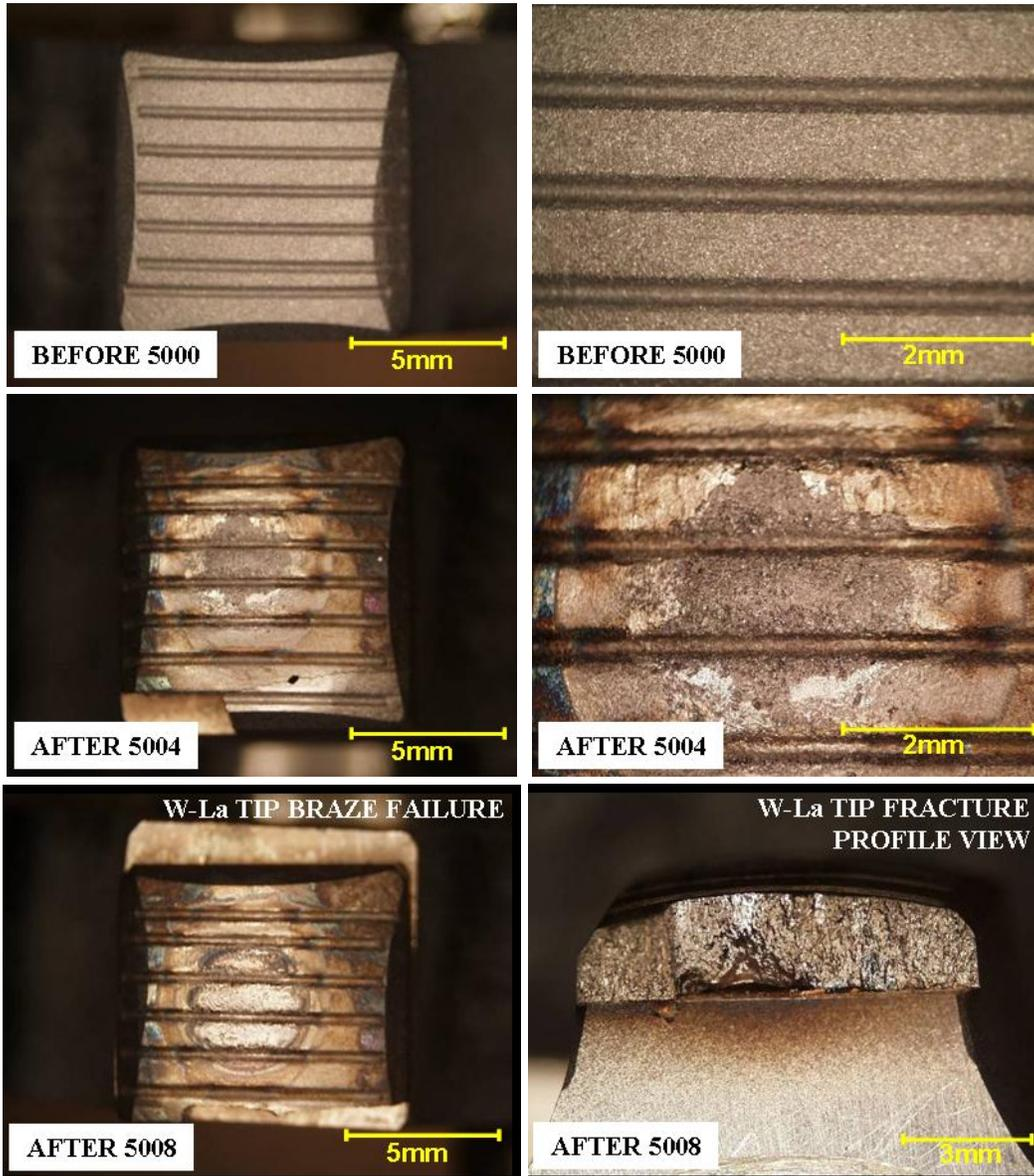
Figure 128: W-La tip after SS 410 weld trials 5000-5008
