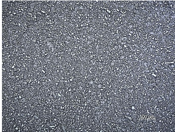
Figure 5: FerroTitanit WFN - martensitic structure with TiC carbides (68 HRC)
