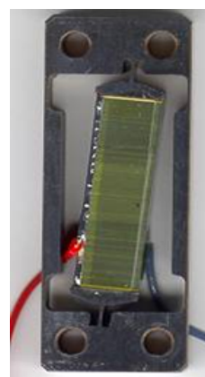
Fig. 2. (Color online) Piezoelectric multilayer actuator with a stroke-amplifying mechanism using flexural hinges [6].
