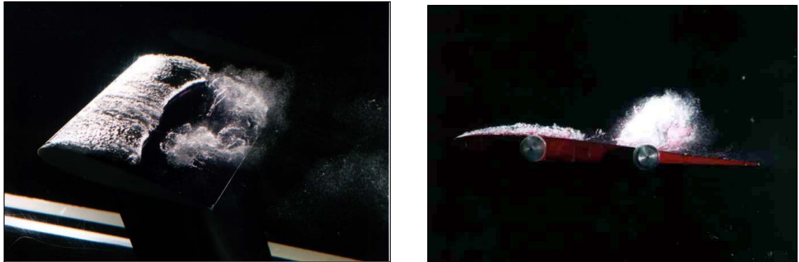
Figure 1.1 - Photographs of cavitation generated by high speed lifting body shapes. [University of Tokyo]
