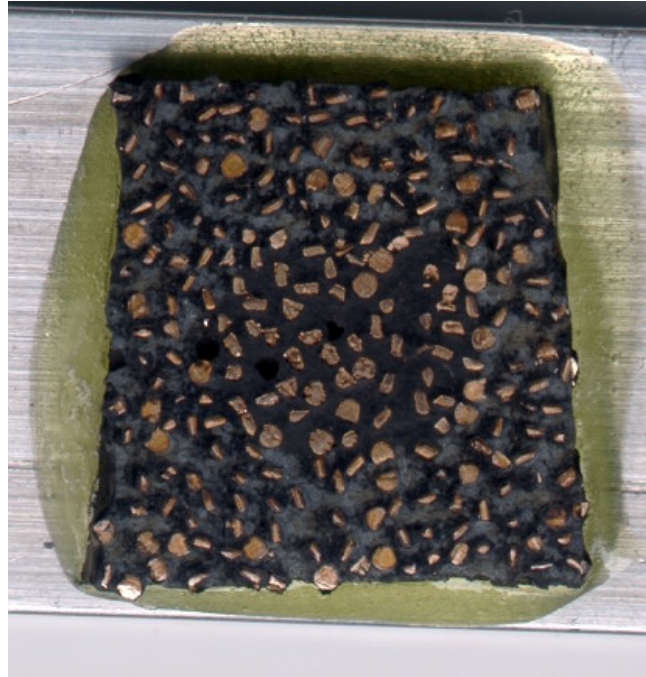
Figure 5.16 – Cuproprene sample showing damage to embedded copper-nickel granules
