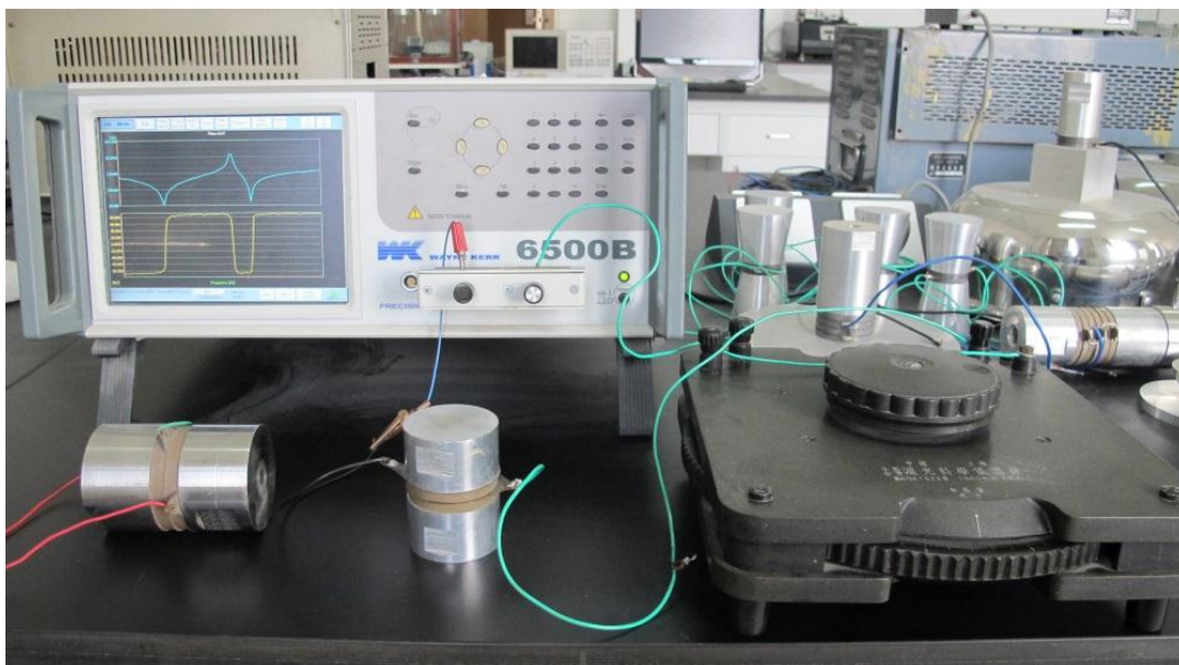
Figure 12. Experimental set-up for the measurement of the frequency response.
