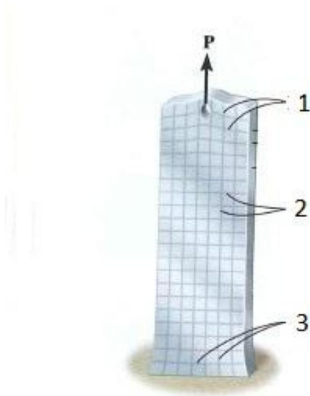
**Figure 2.5** Localized deformation when a force  $P$  is applied on a member. (Figure extracted from reference [22])
