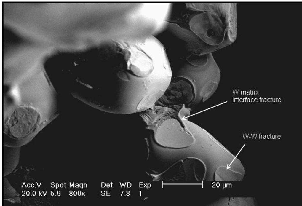
**Figure 4.26** Fracture surface of IT180 at x800 magnification (SEM).
