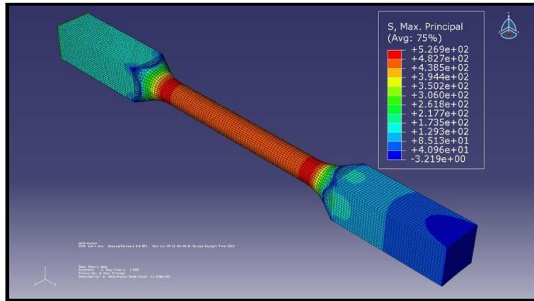
**Figure 4.7** First analysis of specimen stress distribution to the real size model.
