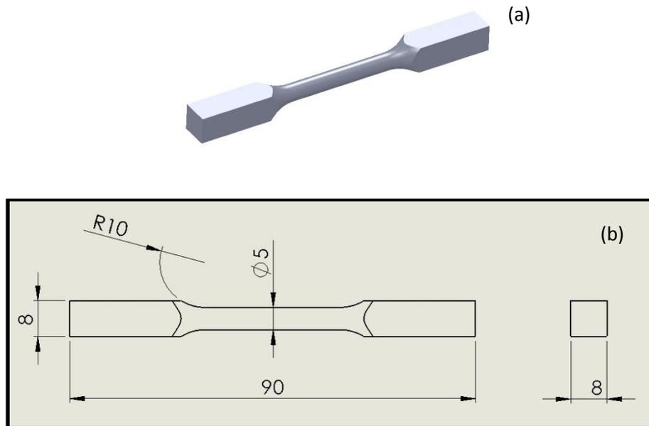
**Figure 3.1** Sample modeled with SolidWorks; (a) 3D view, (b) sample dimensions in mm.
