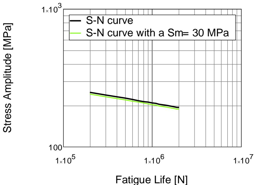
Figure 4.23 Mean stress effect in the *S-N* curve of IT180.
