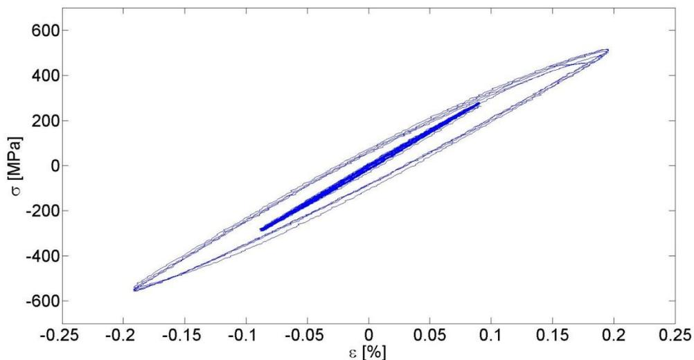
**Figure 4.28** Hysteresis loops for IT180 until 0.2% of strain amplitude.
