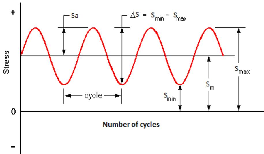
**Figure 2.1** Cyclic stress variation with time and nomenclature for stress parameters which affect fatigue life.
