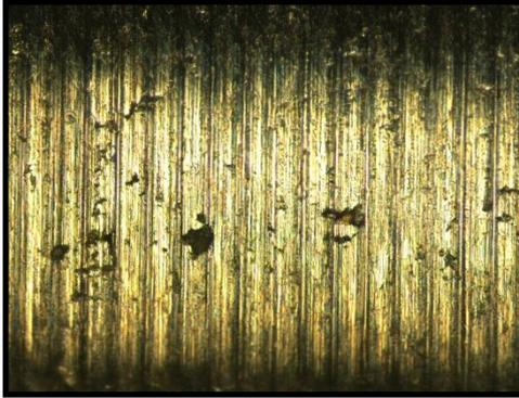
**Figure 4.1** Specific area before grinding and polishing.
