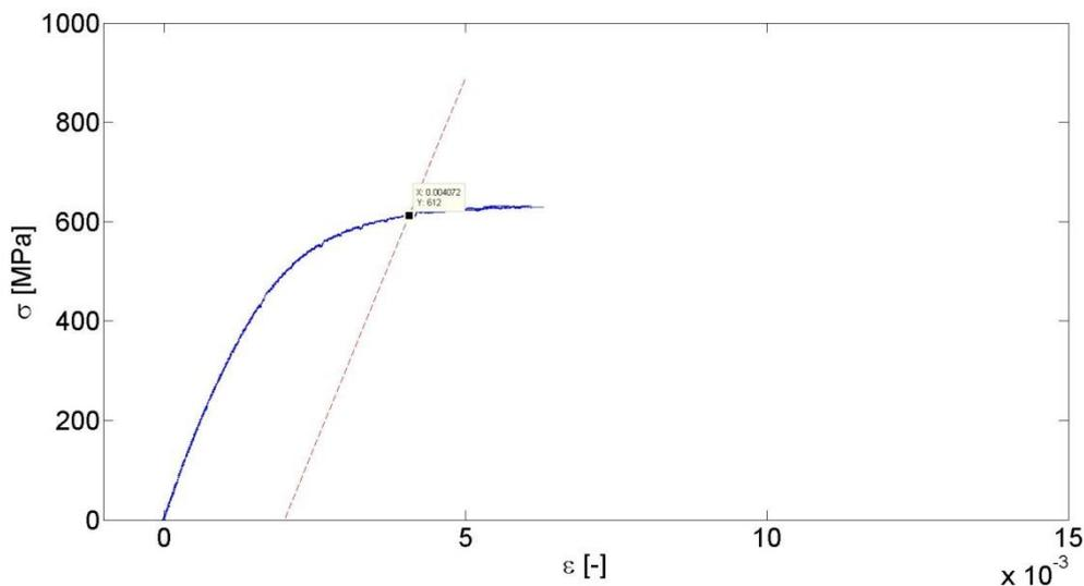
Figure 4.19 Stress vs. Strain diagrams of Inermet 180.
