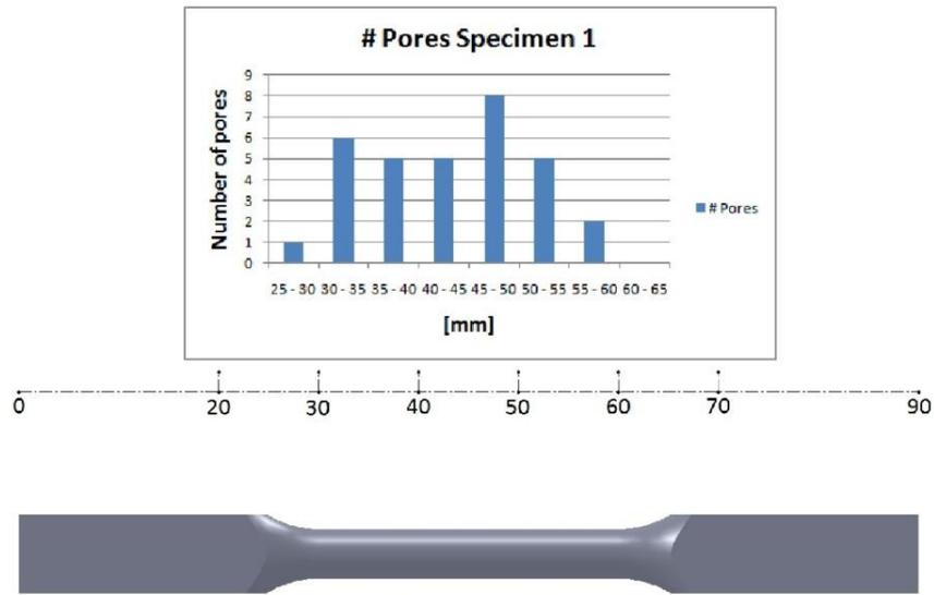
Figure 4.4 Pore distribution along specimen #1.
