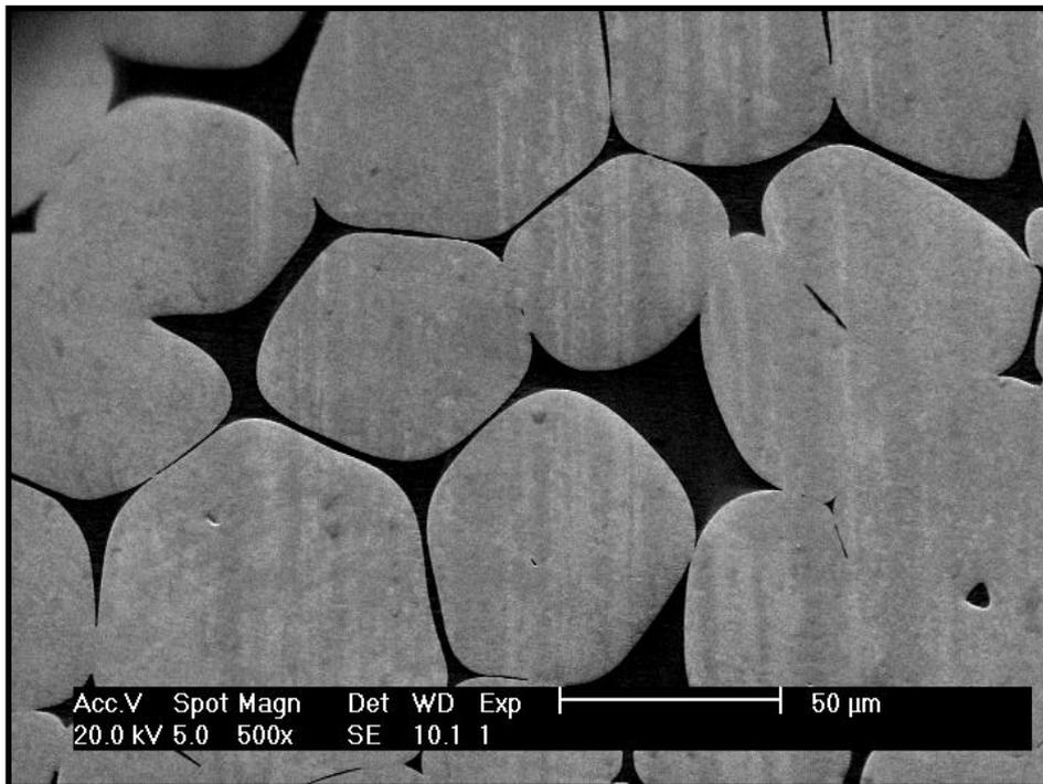
**Figure 4.14** Microstructure of Inermet 180 alloy (SEM magn. x500).
