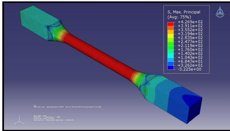
**Figure 4.9** Third FEM analysis, with 20 mm radius model.
