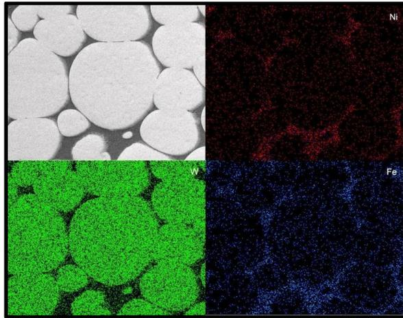
Figure 4.17 X-ray mapping by electron dispersive microscopy of D176.
