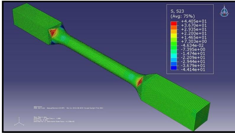
**Figure 4.13** FEM analysis of the first model (10mm blend radius) showing shear stresses  $S_{23}$ .
