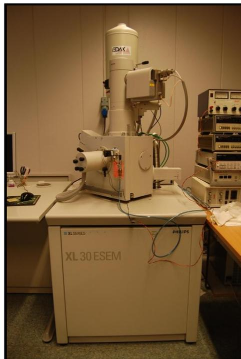
**Figure 3.7** Philips XL 30 ESEM used to study the samples surface and fracture surfaces.
