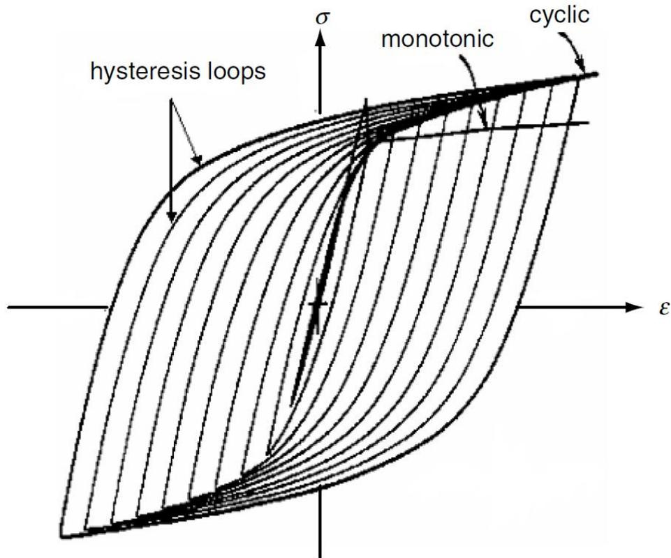
**Fig. 2.3** Hysteresis loops at different strain levels and the cyclic stress-strain curve formed by joining the locus of the loop tips. The tensile curve is superimposed in the figure to show the relationship between the cyclic and monotonic behavior of the material. (Figure extracted from reference [13].)
