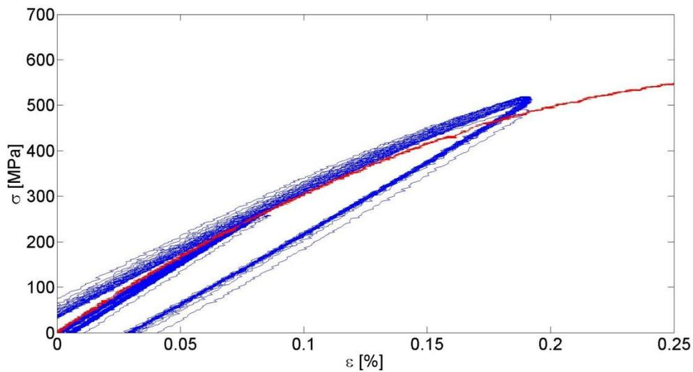
**Figure 4.31** Tensile side of the hysteresis loops for IT180 together with the tensile stress-strain curve.
