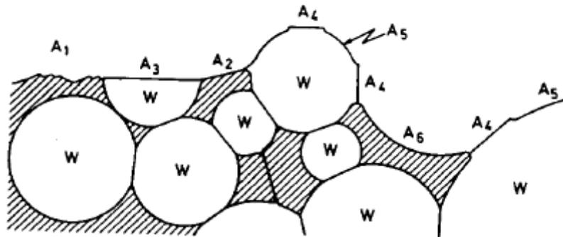
**Figure 4.25** Schematic illustration of major failure modes. A1= ductile fracture of matrix-phase; A2= intergranular fracture of matrix-phase; A3= transgranular cleavage; A4= intergranular fracture of W-grains network; A5= tungsten side of W-matrix interface fracture; A6= matrix side of W-matrix interface fracture. (Picture taken from reference [8].)
