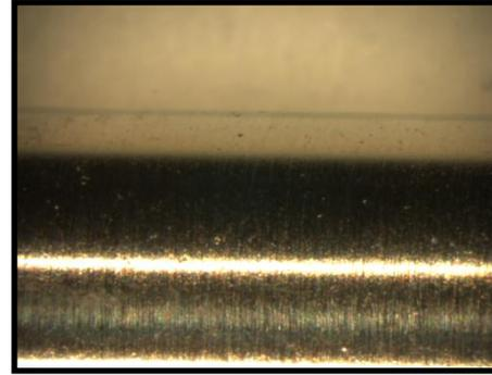
**Figure 3.3** Surface of the IT180 sample seen at x20 magnification after grinding and polishing.
