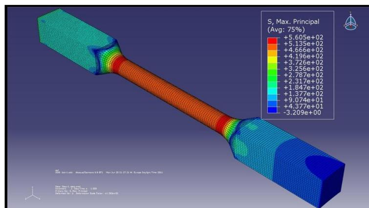
**Figure 4.8** Second FEM analysis, with 8 mm radius model.
