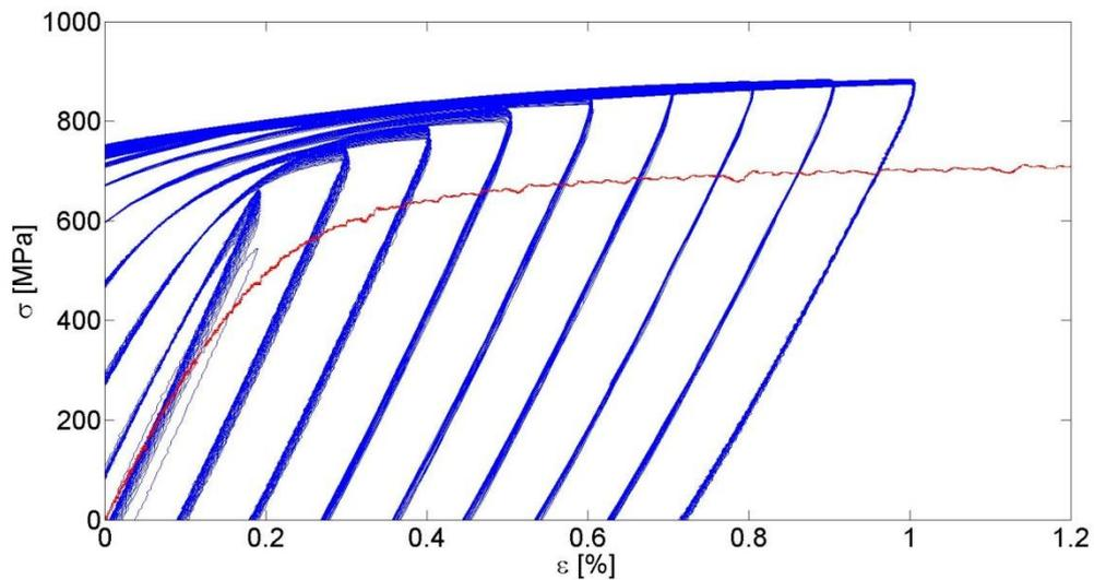
**Figure 4.32** Tensile side of the hysteresis loops for D176 together with the tensile stress-strain curve.
