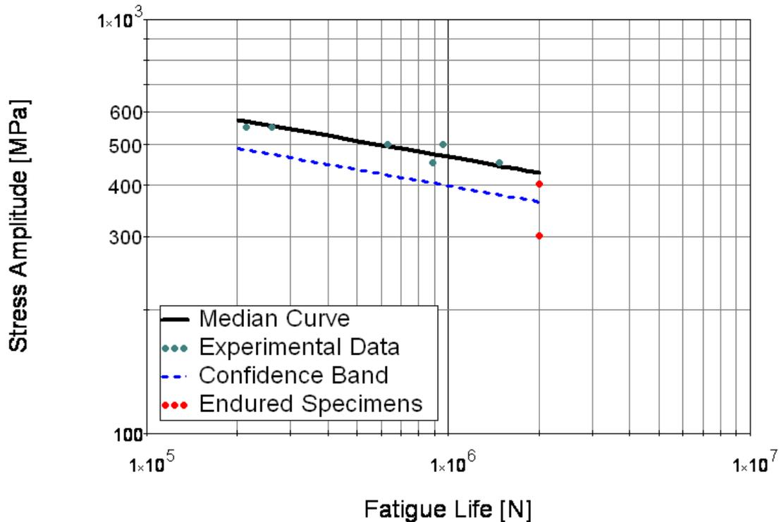
**Figure 4.22** Experimental data of D176 in the finite life region along with the statistical median curve and the confidence band.
