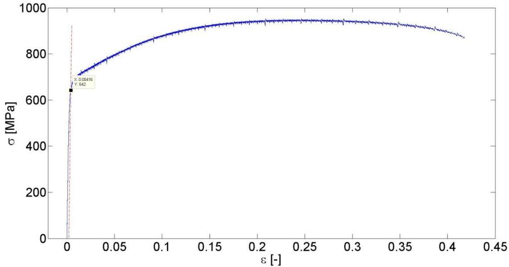
**Figure 4.20** Stress vs. Strain diagrams of Densimet 176.
