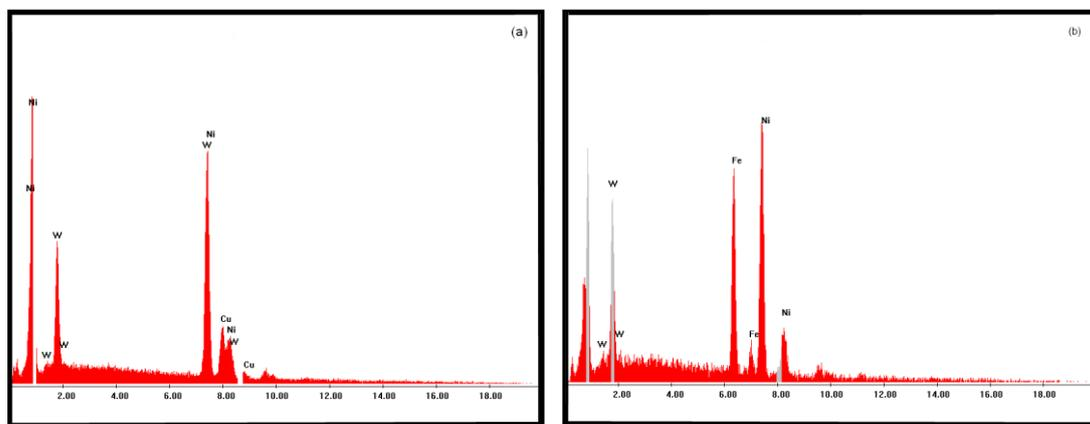
Figure 4.18 Composition analyses in a spot within the ductile phase of each alloy showing (a) Amount of nickel, copper and tungsten in the IT180 matrix and (b) Amount of nickel, iron and tungsten in the D176 matrix. ; Note the high presence of W in the ductile phase of D176.
