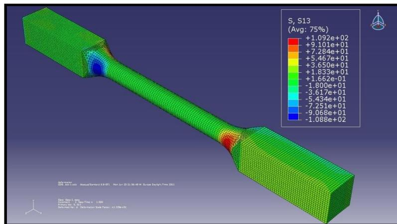
**Figure 4.12** FEM analysis of the first model (10mm blend radius) showing shear stresses  $S_{13}$ .
