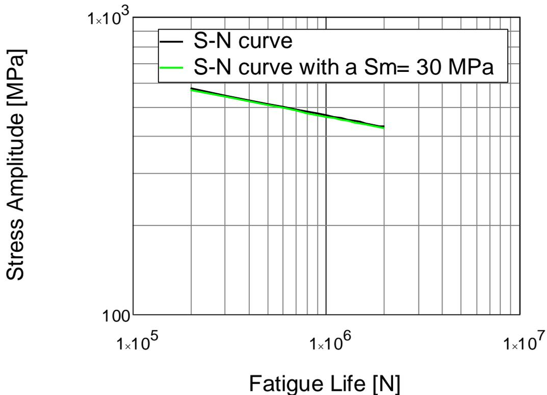
**Figure 4.24** Mean stress effect in the S-N curve of D176.
