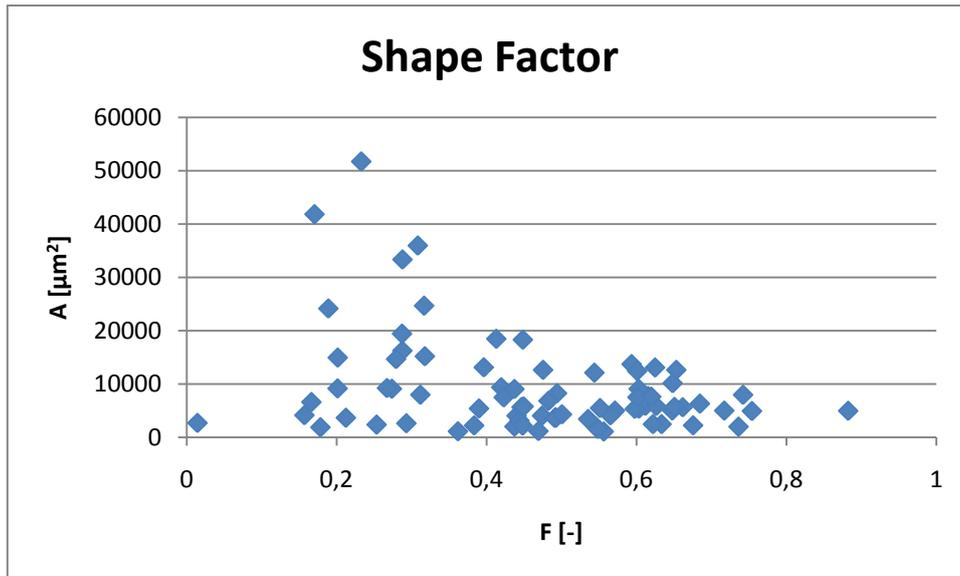
**Figure 4.3** Shape factor calculated for the pores registered in 3 specimens of IT180.
