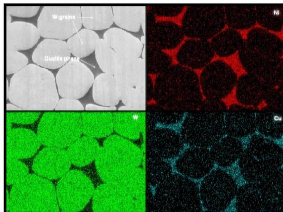
**Figure 4.16** X-ray mapping by electron dispersive microscopy of IT180.
