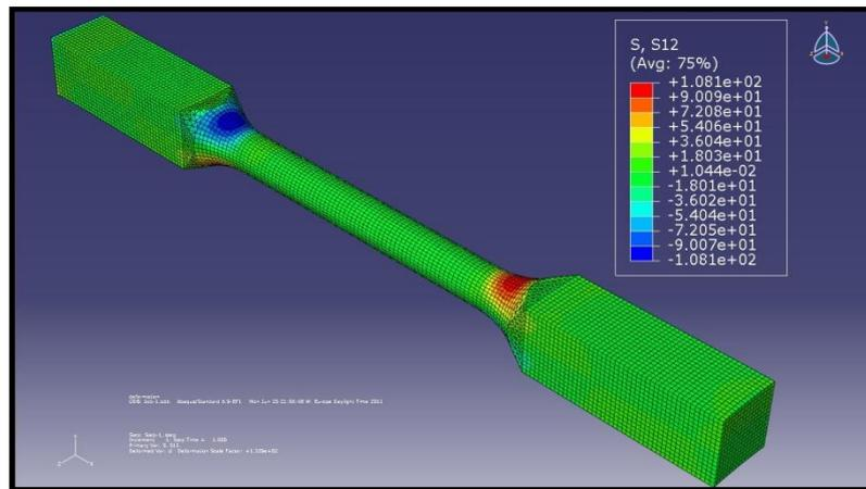
**Figure 4.11** FEM analysis of the first model (10mm blend radius) showing shear stresses  $S_{12}$ .
