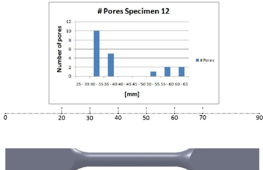
**Figure 4.6** Pore distribution along specimen #12.
