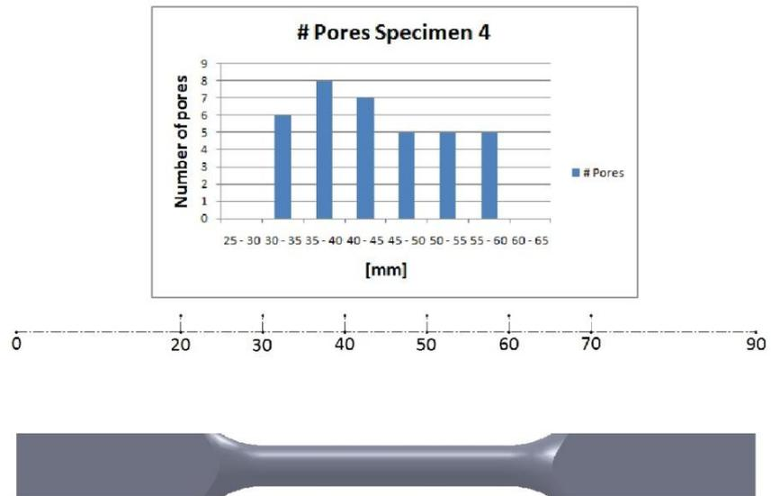
Figure 4.5 Pore distribution along specimen #4.
