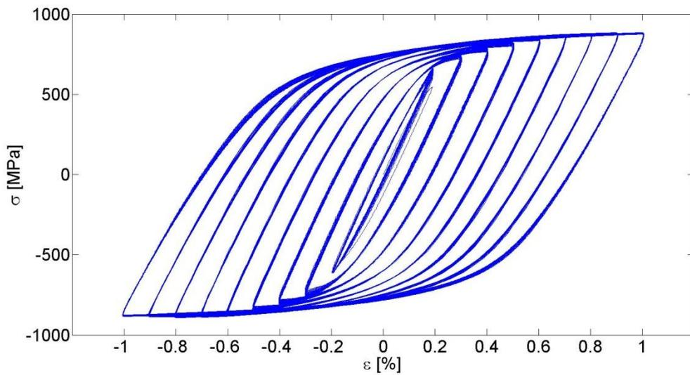
**Figure 4.29** Hysteresis loops for D176 until 1% of strain amplitude.
