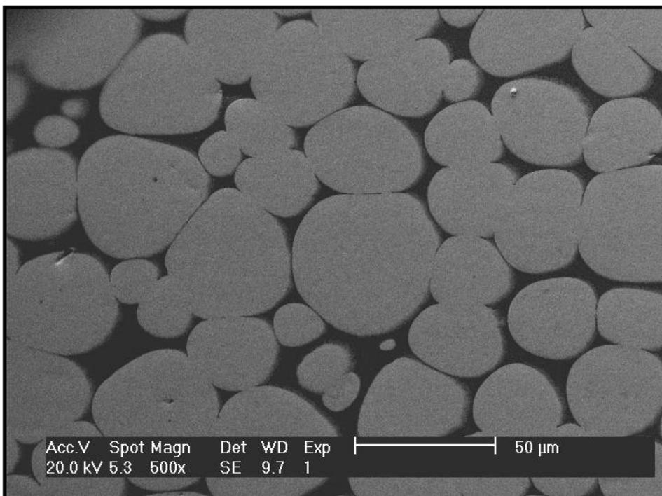
**Figure 4.15** Microstructure of Densimet 176 alloy (SEM magn. x500).
