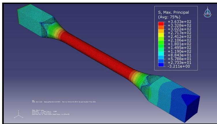
**Figure 4.10** Fourth FEM analysis, with 30 mm radius model.
