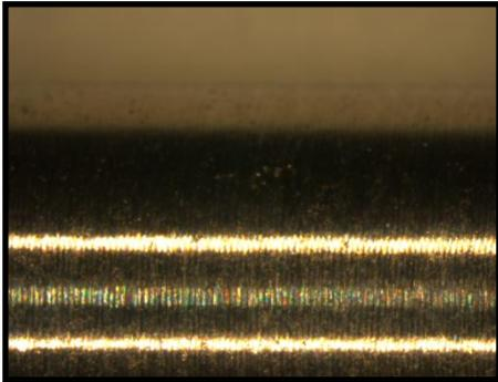
**Figure 3.2** Surface of the IT180 sample seen at x20 magnification before grinding and polishing.
