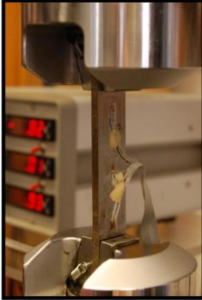
**Figure 3.9** Metal piece with sensors used to align the specimen.
