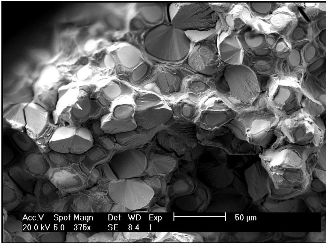
**Figure 4.27** Fracture surface of D176 at x375 magnification (SEM).
