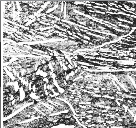
BLOCKY ALPHA WITH GRAIN BOUNDARY ALPHA DECORATING PRIOR BETA GRAIN BOUNDARIES
