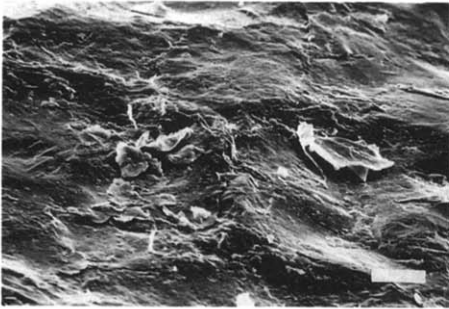
Fig. 2. Surface topography of shot-peened pure iron. Marker 50 \mu\text{m} .
