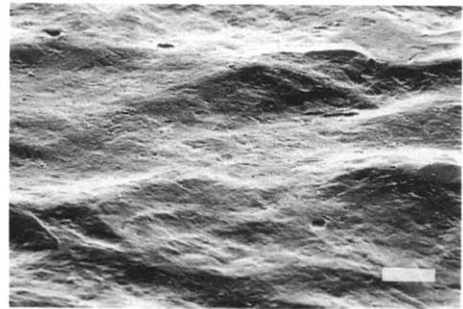
Fig. 2. Surface topography of shot-peened pure iron. Marker 50 \mu\text{m} .
