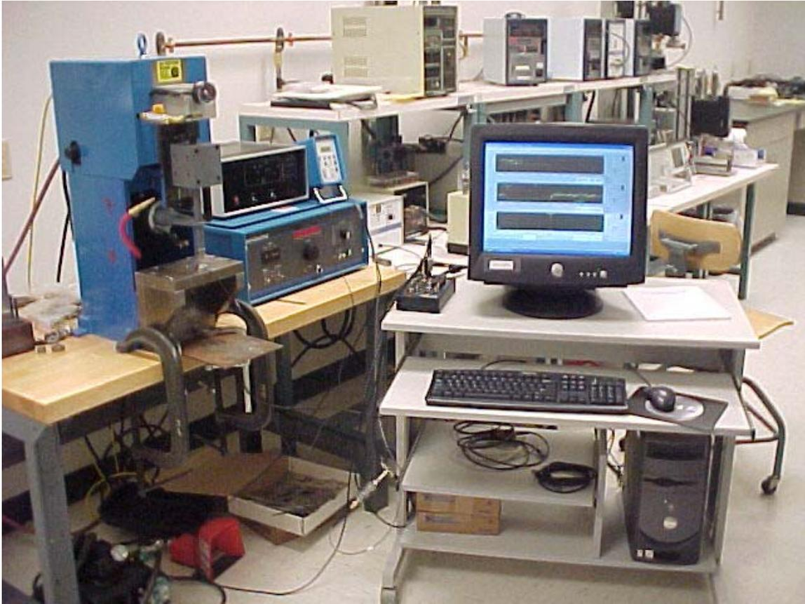
**Figure 5.6: Ultrasonic welding system and DAQ.**
