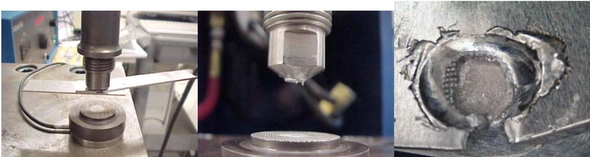
**Figure 6.58: Sonotrode welded to the top part and extrusion for anti-resonant top part weld.**
